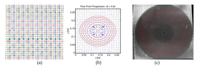
**Figure 2:** Output results; (a) section of textile geometry identified using image analysis techniques, (b) Predicted flow front evolution from predicted permeability map and (c) actual flow front evolution observed
